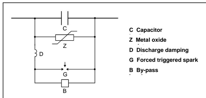
Fig. 4: Main configuration of a Series Capacitor.
